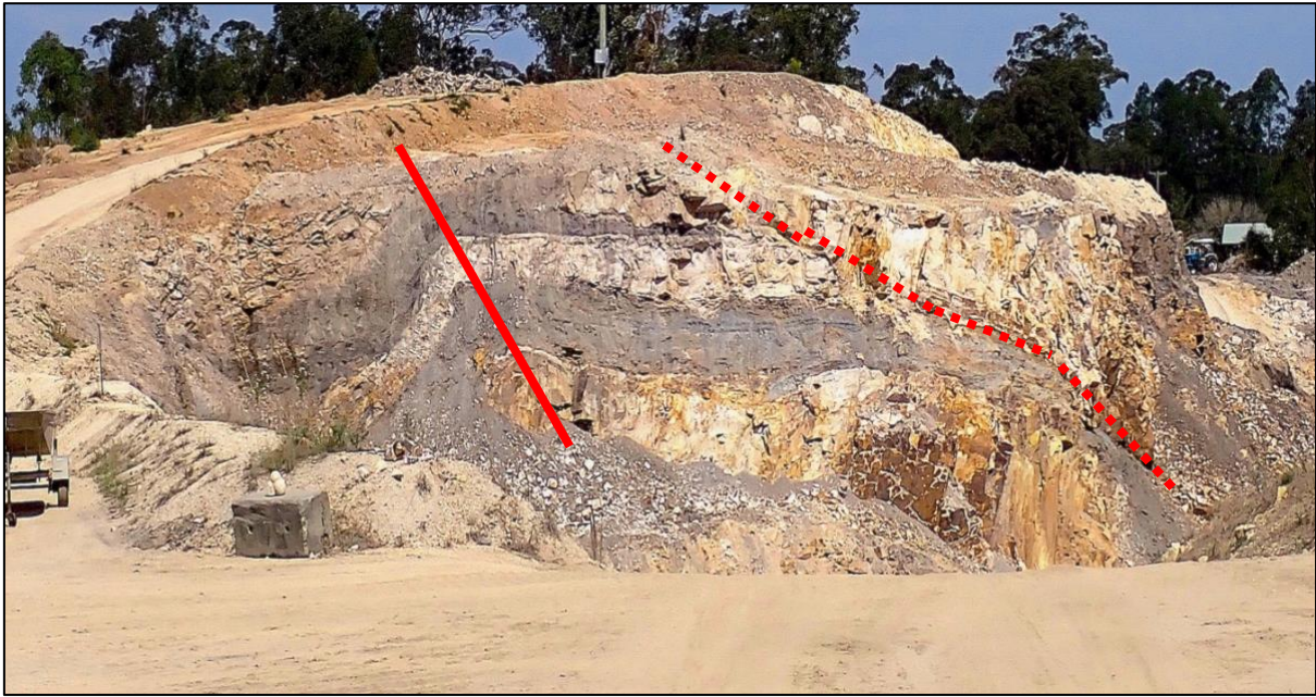
Photo 10. The southern quarry face in September 2024 showing the exposed structures and stratigraphy. Chris Morton photo. Fold axis: ——— Thrust fault: - - - - -
