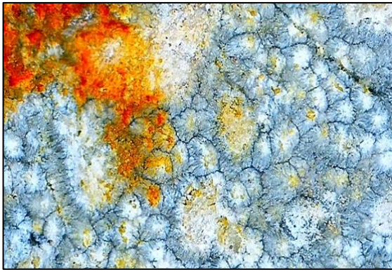
Photo 27. Devitrified glass (vitrophyre) comprising feathery white crystallites. Photomicrograph by Chris Morton. Field of view is 0.5mm.
